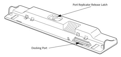
Figure 4-17 Port Replicator front panel
