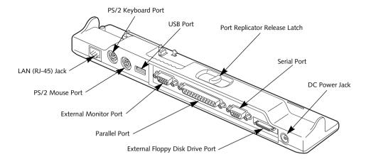
Figure 4-16 Port Replicator rear panel
