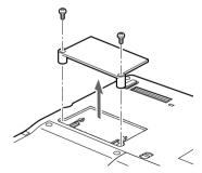
Figure 4-13 Opening the Memory Upgrade Compartment
