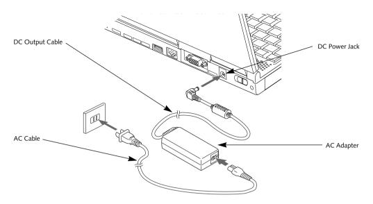
Figure 3-1 Connecting the AC Adapter
