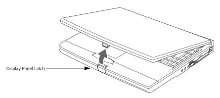
Figure 3-2 Opening the Display Panel
