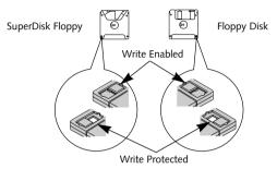
Figure 4-5 Floppy Disk Write Protect
