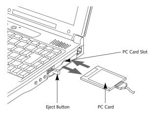
Figure 4-12 Installing/Removing PC Cards
