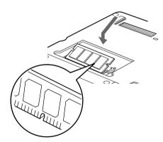
Figure 4-14 Installing a Memory Upgrade Module
