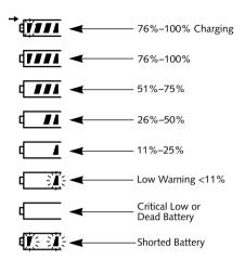
Figure 2-11 Battery Level Indicator
