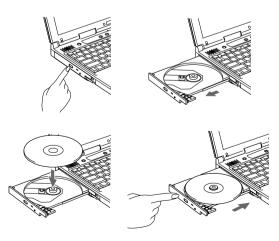
Figure 4-7 Loading/Ejecting a CD
