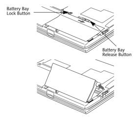
Figure 4-1 Replacing the Battery
