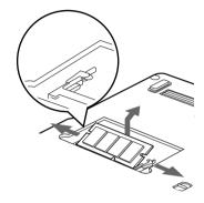
Figure 4-15 Removing a Memory Upgrade Module
