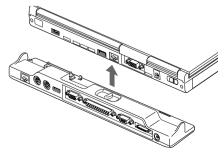
Figure 4-18 Attaching the Port Replicator
