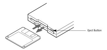
Figure 4-2 Loading/Ejecting a 3.5" Floppy Disk
