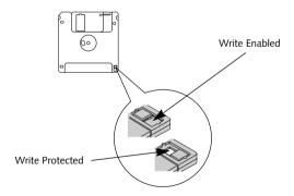
Figure 4-3 Floppy Disk Write Protect
