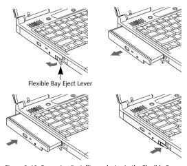
Figure 2-19 Removing/Installing a device in the Flexible Bay
