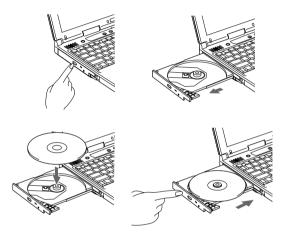
Figure 4-10 Loading/Ejecting a DVD/CD
