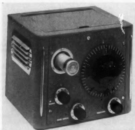
This "super-selective converter" is a complete receiver front end plus a two-stage 1525-kc. crystal lattice filter. It is intended to work ahead of any receiver capable of tuning to 1525 kc. The oscillator coil is plug-in, at the upper left.
